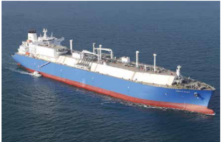
Figure 5. Teekay's Creole Spirit LNG carrier powered by a MAN ME-GI engine (Courtesy of Teekay LNG Partners)
